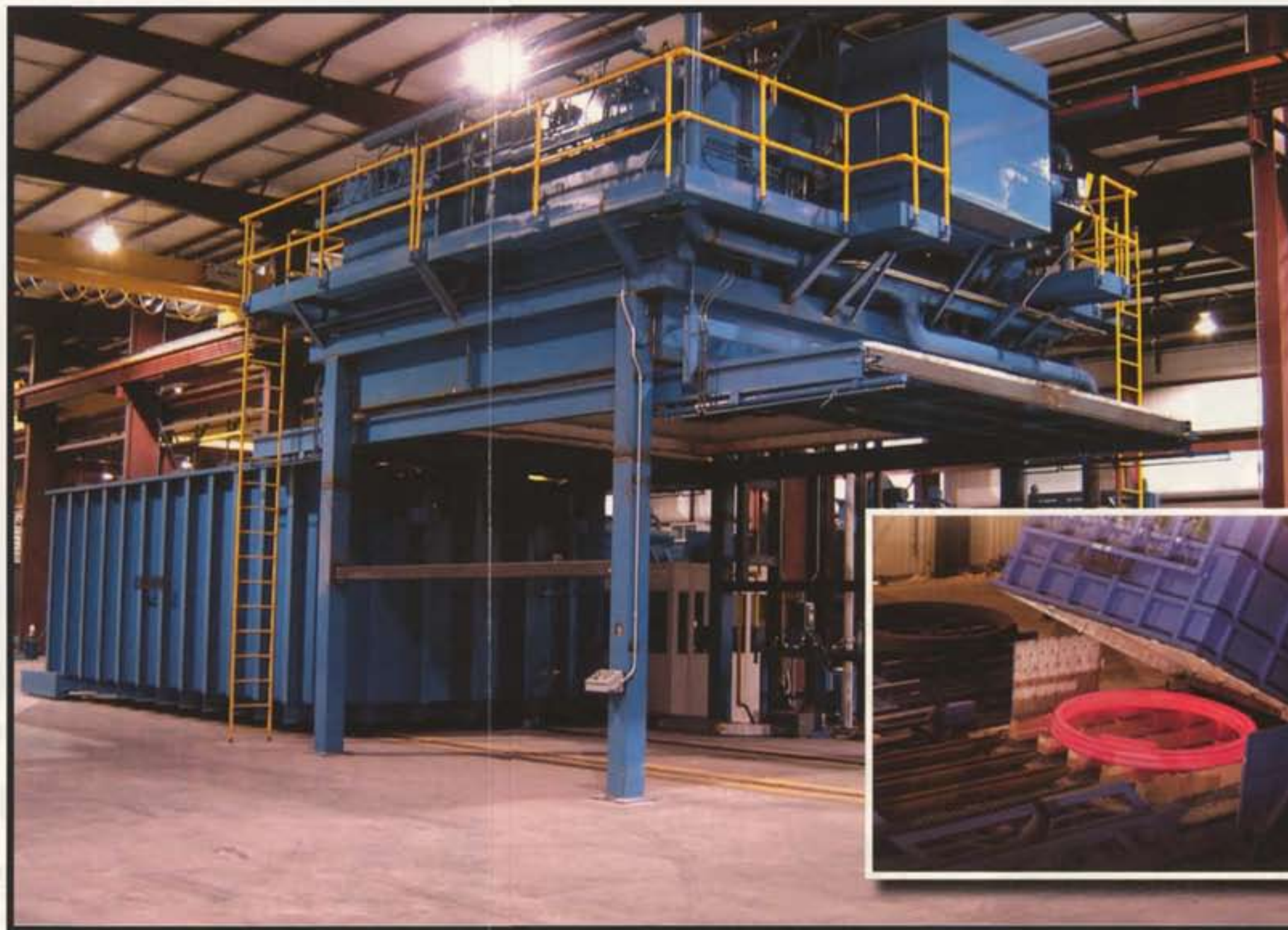
This aluminum drop bottom furnace (left) has a working zone of 174x174x48 inches. It can accommodate an 8,000-lb load capacity, and has rapid quench capability via drop bottom quench into a 19,000-gal water tank.
