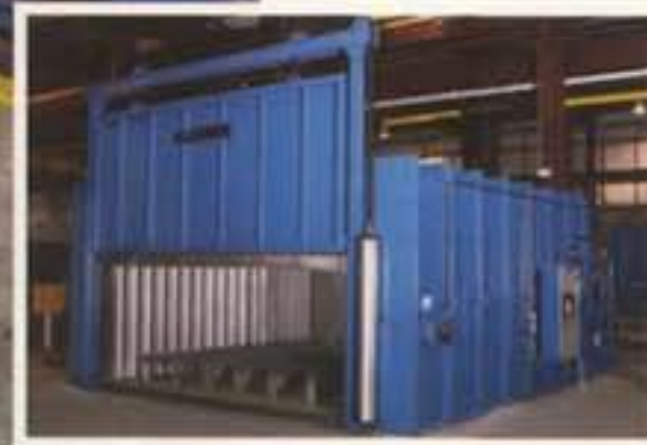
This aluminum aging oven is designed to operate in a temperature range of 170°-600°F
