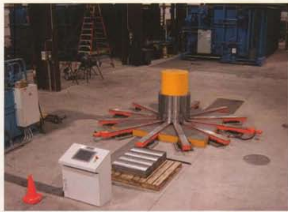
SII's new ring expander (top) has a 5-in. stroke with a 12-segment expansion head. It has an ID capability of 32- to 136x30 inches high.
